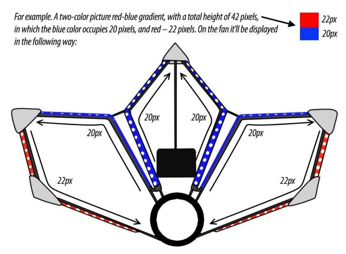
The arrows inside the fan show the guide paths how the picture is bent and displayed. If you hold a "pixel poi" and not a fan, it'll display the picture straight. But in this case, on the sideward rays where the red color is, the picture bends downward. That's why in the example, the upper red 22 pixels will bend down on the sideward "crystals".
